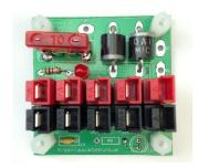
Cut the remaining piece of thick wire into **two equal pieces** and install them in the positions marked **N** and **R**.
